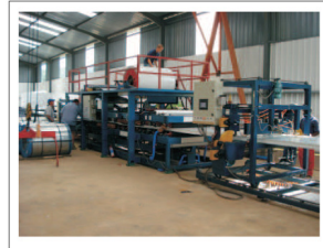
SIPS Panel Plant
