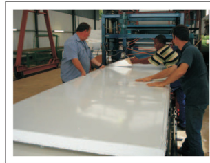
Panel cut to length
